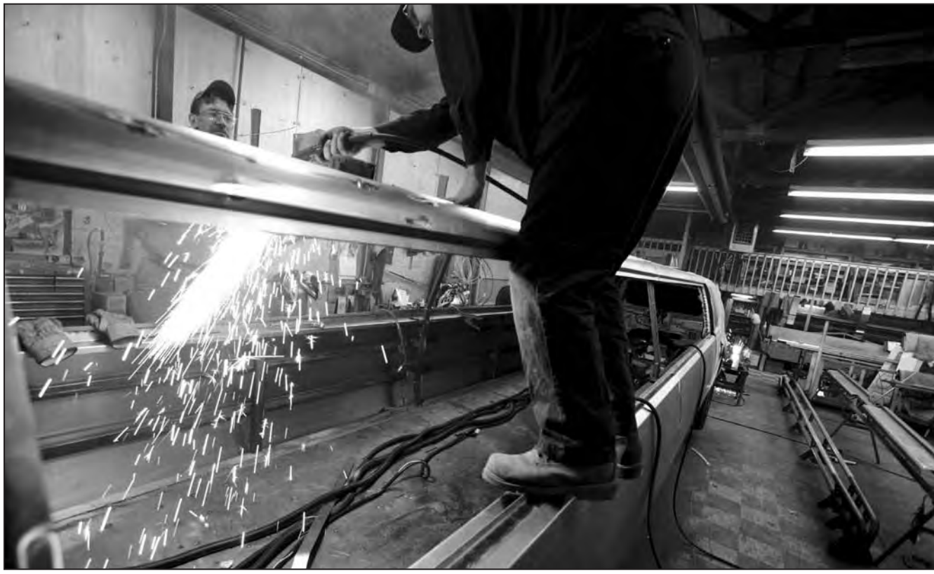
Mike Frantz cuts a moon roof into a Cadillac Escalade stretch limo being built at Great Lakes Limo in Forester, Mich.
