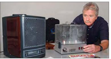
Mike Whittemore demonstrates how the Living Proof unit ionizes smoke particles, causing them to clump together magnetically and settle to the floor.
