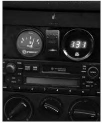
The Floeser's 2001 Jetta, which has been retro-fitted to run on vegetable oil, has a panel with a gauge (left), showing the amount of vegetable oil in the tank; a switch in the middle to change from diesel to vegetable oil (center) and a gauge that measures the temperature of the vegetable oil.
