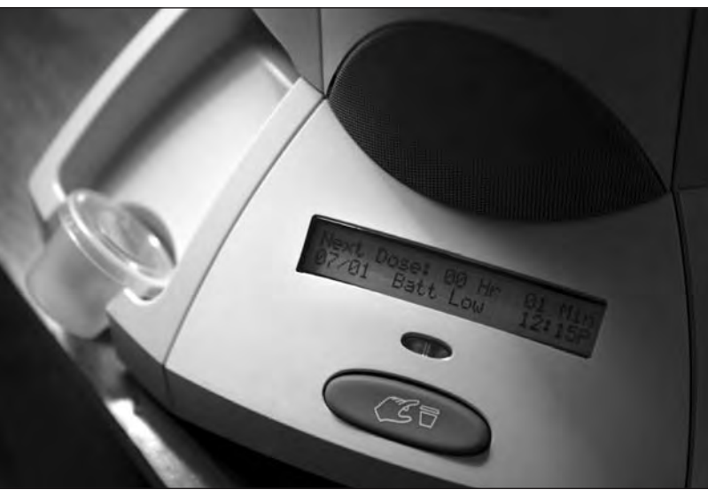
AssuraSource has installed a pill-dispensing machine that reminds seniors to take their medication. If they don't, the machine is linked to a phone so it can notify the company's nurse to call and check on them.
