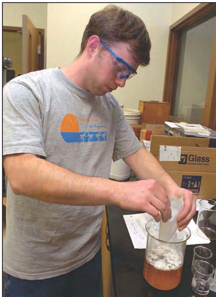
WVU Biodiesel Project President Lucas Ellis separates glycerol from the biodiesel before starting an experiment.
