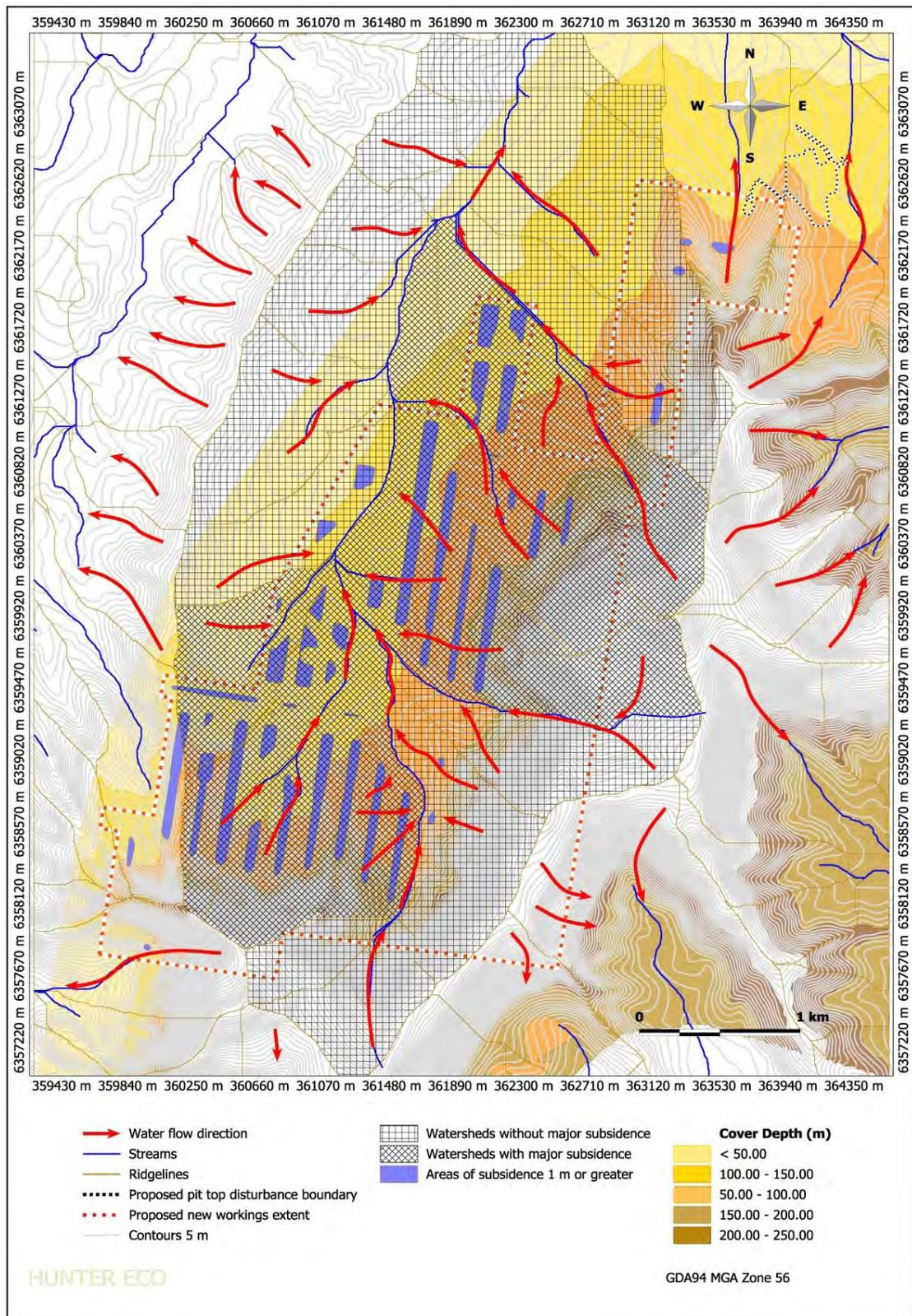
Figure 7 Catchments subjected to subsidence and cover depth
