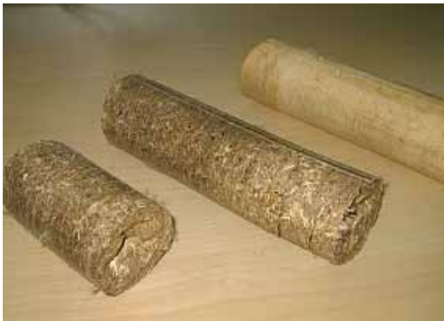
Reed briquettes on left and middle, wood briquette on right. Photo: Teemu Kettunen.
