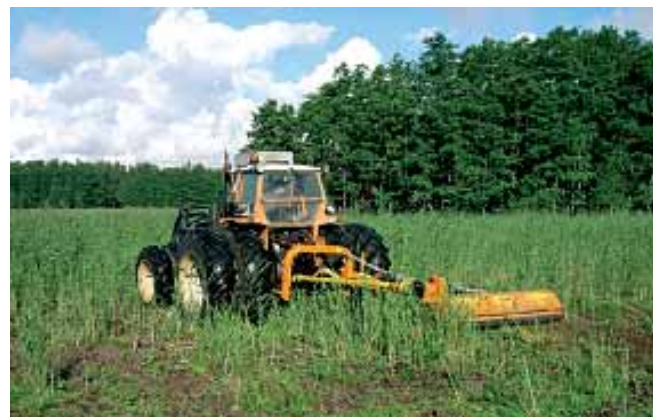
Picture 3. The wider 2.2 m crusher attached to the back of a tractor. Photo: Ilpo Huolman.
