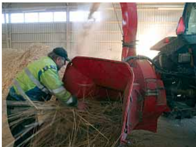
Chipping dry reed for burning tests in Halikko, Finland, in May 2007. Reed can be very viscous, and it can be difficult to chip it into very small pieces (under 5 cm) with the common wood chipping machinery. Photo: Eija Hagelberg.
