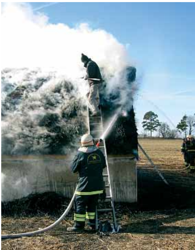
While burning, the reed roof is covered in thick smoke. In this 1:1 burning test, a fireproof fabric has been used on the roof. Photo: Carlo F. Christensen.
