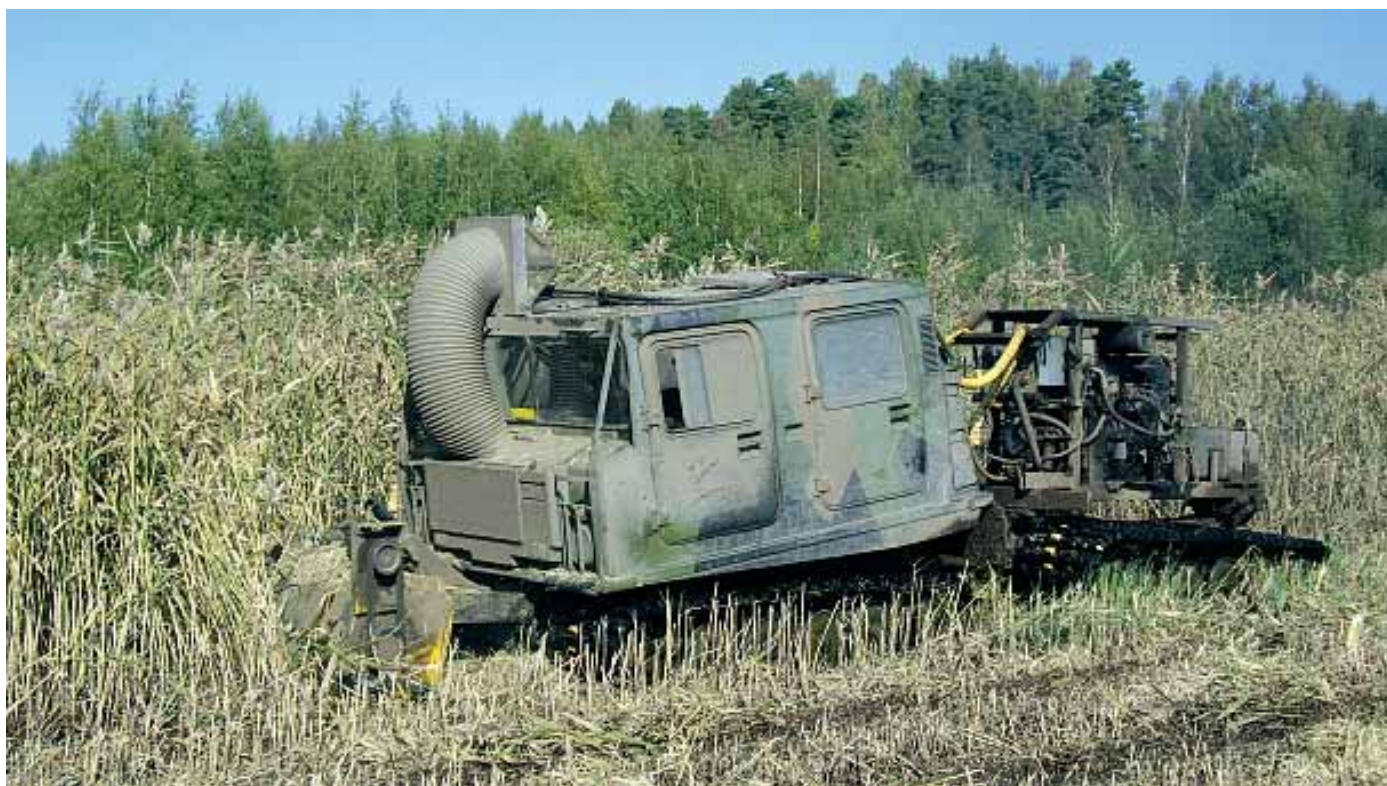
Picture 4. A narrow 1.6 m crusher attached to a lorry with caterpillar tracks (Hägglund BV 206). Photo: Ilpo Huolman.
