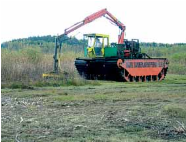
Picture 5. Equipment on caterpillar tracks can be used to cut meadows even in the softest of terrains. Photo: Ilpo Huolman.
