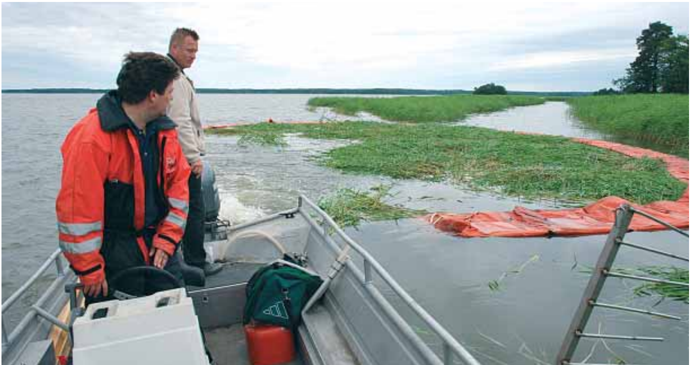
Cutting reed with a boat-mounted mowing machine is a quick job, but gathering in the cut material is another matter. This is a test to gather mowed reed using surface oil dispersal booms in Mietoinen, Finland, in June 2007. This boom system was a little bit too heavy-handed. Photo: Helena Särkijärvi.
