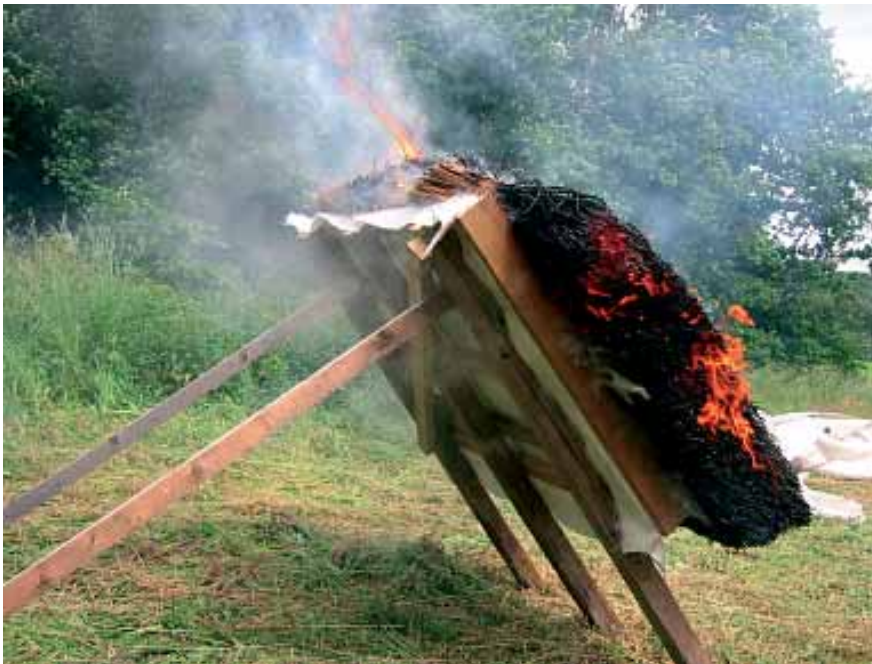
A burning test with a small reed-roof model. Photo: Carlo F. Christensen.
