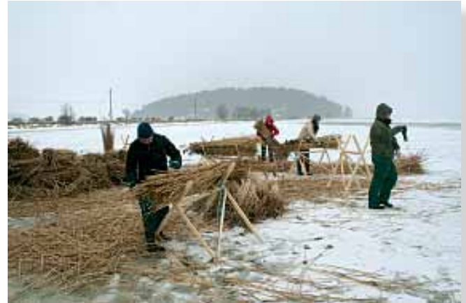
Cleaning bundles of reed takes a lot of work by hand. Course participants in action in April 2006, Salo, Finland. Photo: Eija Hagelberg.
