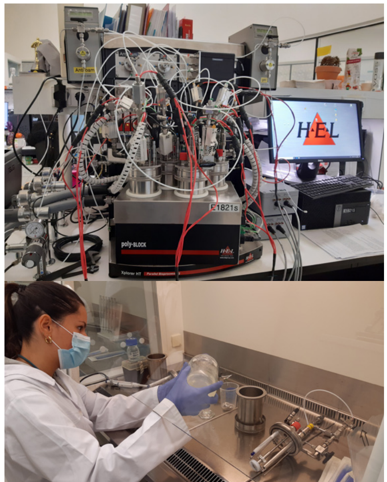
Figure 1 (top). High-pressure bioreactors for the experimental work with deep-sea bacterial isolates. Figure 2 (bottom). Leonor Pizarro (MSc student) preparing the bioreactors for inoculation with a piezotolerant strain.
