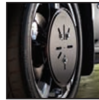
Bolt the Plate to the face of the wheel
