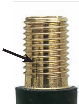
Cracks or cross threads
