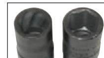
Double Duty - Hex Socket on one end and Twist Socket on the other.
