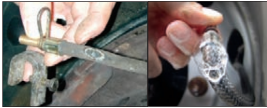
Conventional extensions hold the full air pressure in the extension chamber. Damage to the extension through wear or accident may mean the loss of a tire
