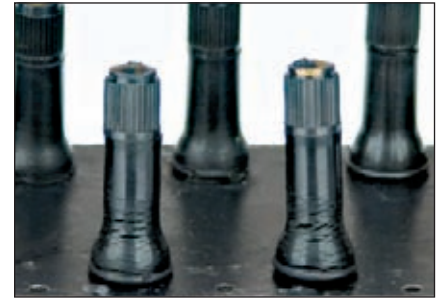
Typically, ozone damage or cracks are seen in low cost valves
