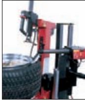
Bead depressing tool aids in demounting
