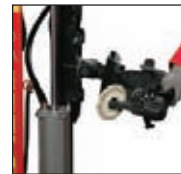
Roller loosens the upper & lower beads
