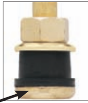
Inspect brass for cracks
