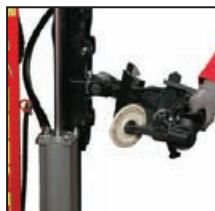
Dual bead breakers work in unison to speed the operation
