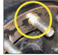
Corrected with centering sleeve
