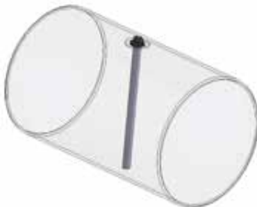
Cross section of round fuel tank w/ Ultimate Fuel Sender
