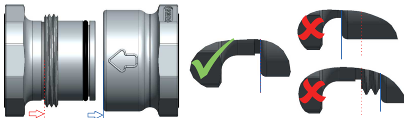
Fig. 40: Verifying the alignment
