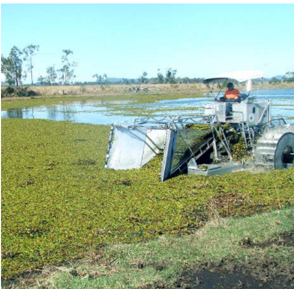
Mechanical harvesting, Mynumai Lagoon
