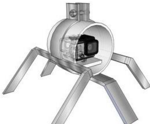
Figure 5 Design of the Rapid Unbaited Drop (RUD) camera, consisting of two opposite facing GoPro cameras
