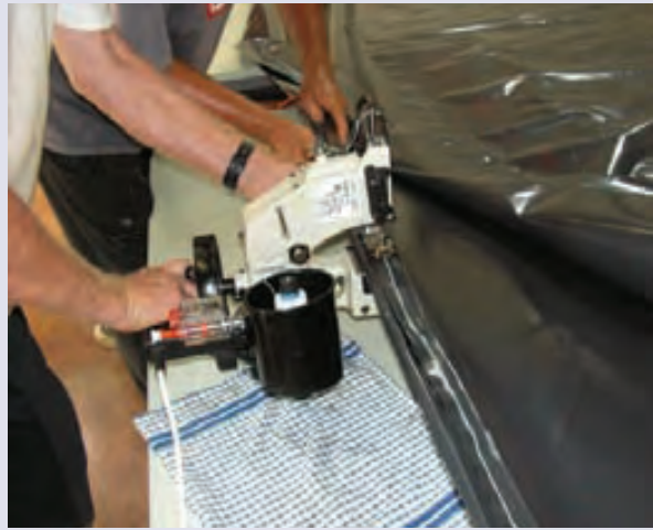
A bag stitcher was used to sew rope into the edges of the plastic.
