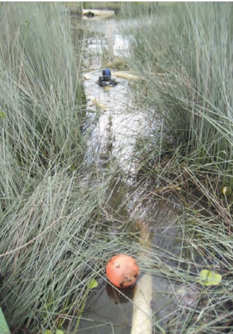
The suction-dredge enables divers to target cabomba in amongst other vegetation.
