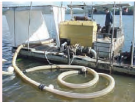
Divers use the suction hose to remove the cabomba including the root ball.
