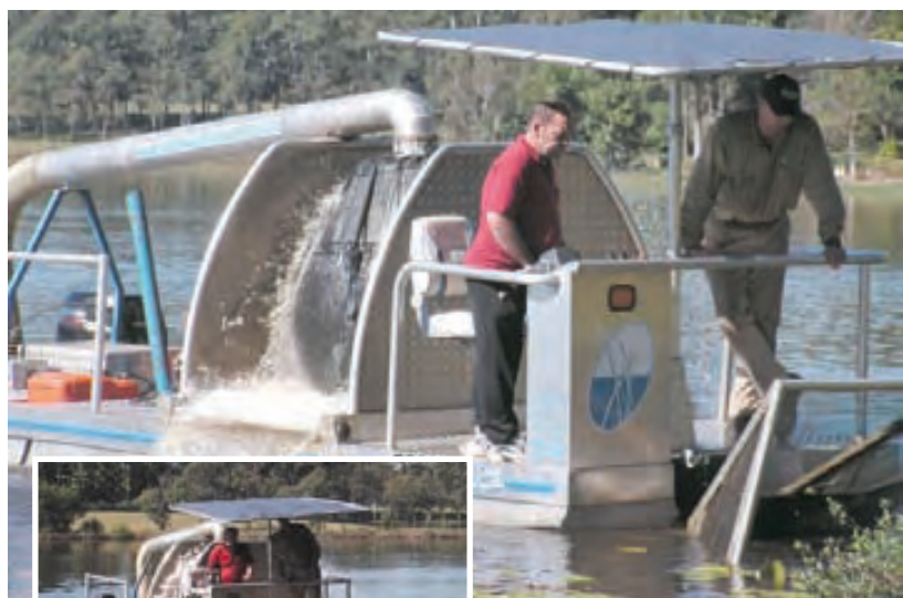
Suction-based harvesters cut and suck cabomba into an onboard bag.
