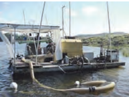
Divers use the suction hose to remove the cabomba including the root ball.
