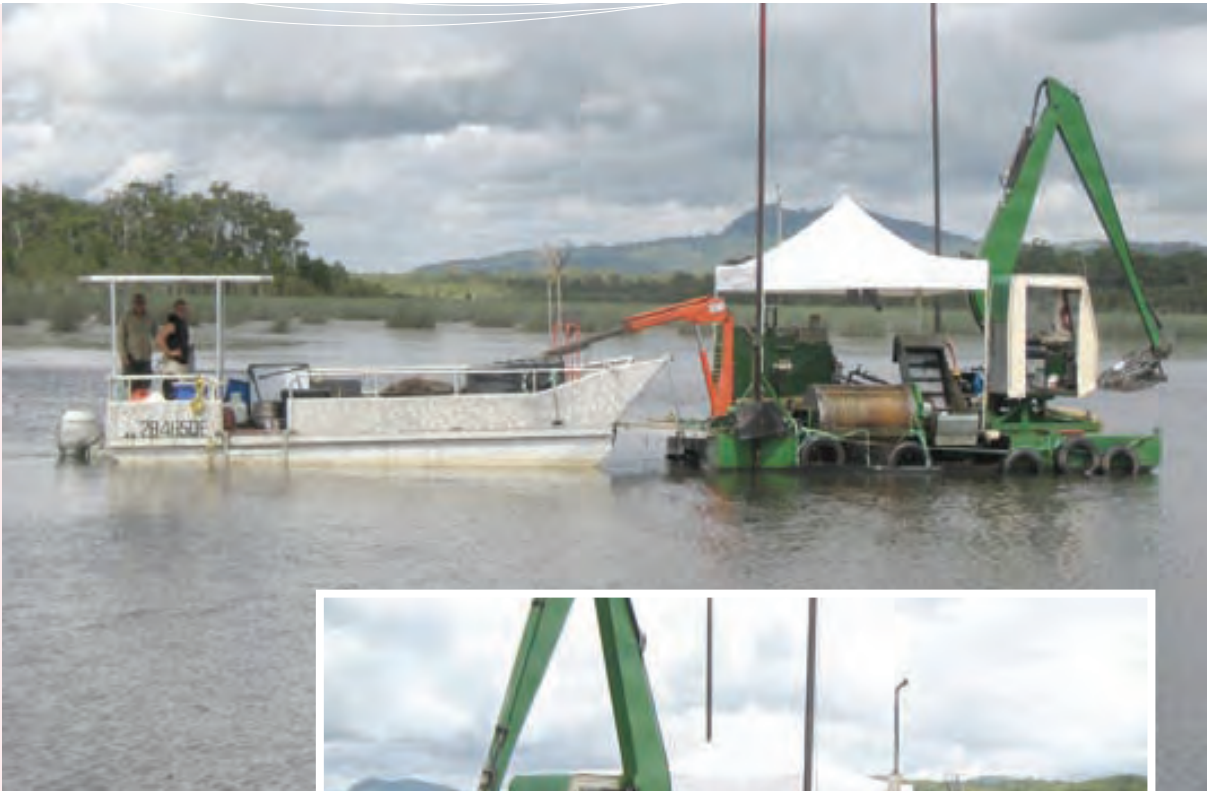
The diver-operated venturi suction dredge
