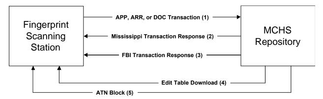
The diagram above shows the flow of information between a fingerprint scanning station (livescan or cardscan) and MCHS. The primary flow consists of a scanning station sending applicant (APP), arrest (ARR), or Department of Corrections (DOC) tenprint transactions (labeled (1) in the diagram) to MCHS and then receiving Mississippi Transaction Responses (labeled (2) in the diagram) and FBI Transaction Responses (labeled (3) in the diagram).
