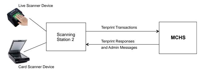
Some requirements in this document are unique to one type of scanning station or another. The single scanning station is responsible for ensuring that all transactions it submits to MCHS (Section 4.1) are compliant with the ICD requirements for each type of scanner device and for handling responses and administrative messages (Sections 4.2 and 4.3).
