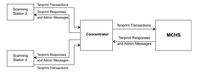
In this configuration, the concentrator is responsible for receiving transactions sent from scanning stations 3 and 4 and sending them to MCHS. Each scanning station has one scanner device attached to it. The concentrator is also responsible for routing all responses from MCHS to the scanning station that generated the corresponding transaction (or to some other appropriate destination).
