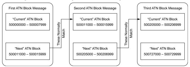
First ATN Block Message: When a livescan is initially set up, the CIC creates and sends the <u>first</u> ATN Block message. This contains the following:
