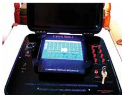
Field portable laser firing unit for laser detonator type I (8 channels)
