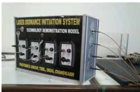
Lab demonstration unit for firing of laser detonator type II (4 channels)
