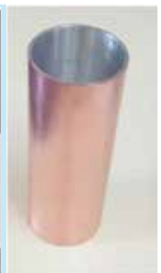
Cu (outer)-Al (inside) cylindrical joint
