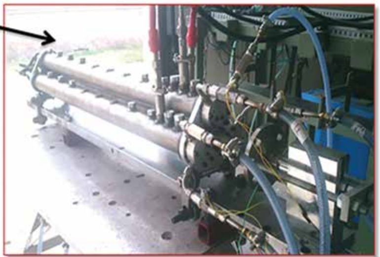
Three tube assembly for PDE system with operating frequency of 24 Hz
