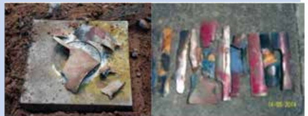
Witness plate after trial and large pieces of casing
