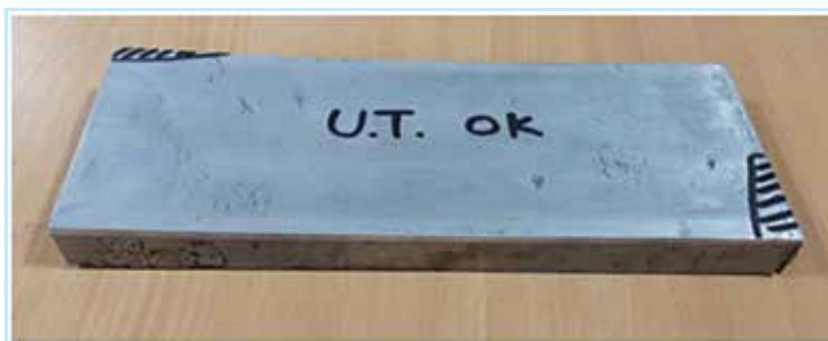
Aluminum (Top) joined to stainless steel (bottom)
