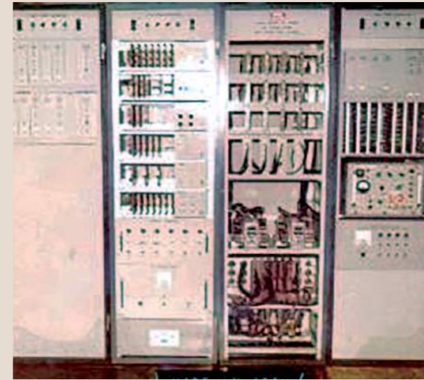
A very large room of vacuum tube electronics re-designed and miniaturised into two racks
