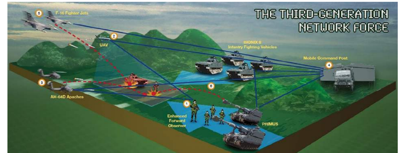
An illustration of IKC2 operations, with the numerical sequence broadly showing how a network of sensors (1 and 2) and shooters (3, 5 and 6) collaboratively locate and defeat targets of interest, with a command post (4) providing oversight.
