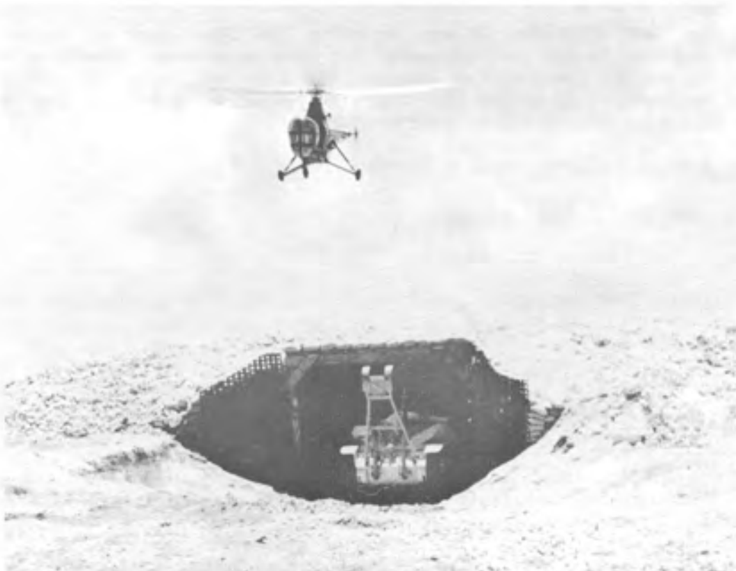
Figure 40. Drone tank in revetment; helicopter hovers overhead to control tank after it has been started, Operation SANDSTONE.
