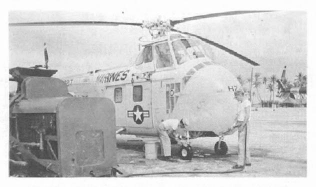
Figure 29. Scrubbing helicopter to remove contamination, REDWING.
