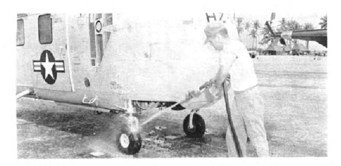
Figure 30. Removing radioactivity from a helicopter, REDWING.
