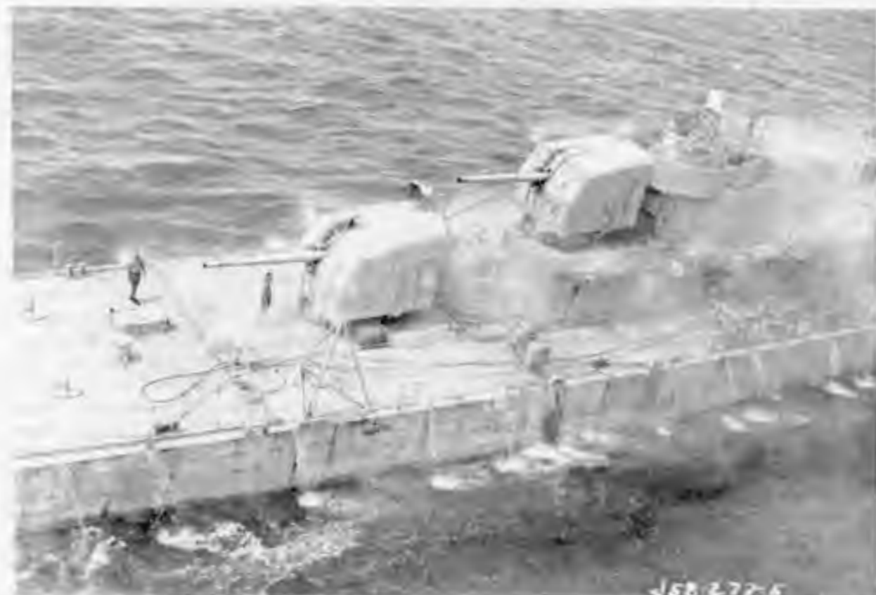
Figure 27. Washdown system operating on rear turrets of Killen (DD-593) during preparations for HARDTACK, UMBRELLA.
