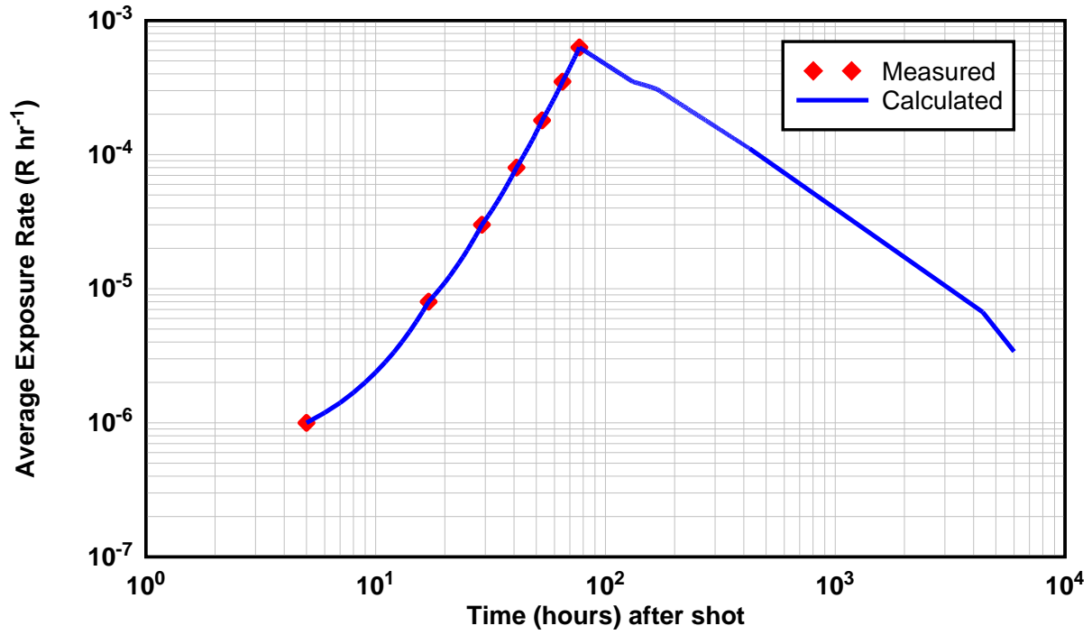
Figure 1. Average Topside Residual Radiation Exposure Rate on USS LIPAN following both Waves of Fallout from Shot MIKE
