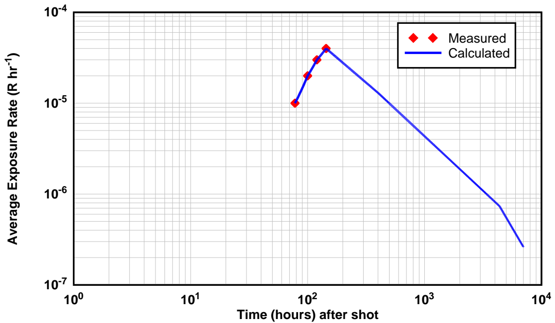
Figure 3. Average Topside Residual Exposure Rate on USS HENRY W. TUCKER from Shot ZEBRA
