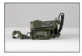
AN/PDR-77 Radiac with Beta/Gamma (β/γ) Probe (DT-616)
