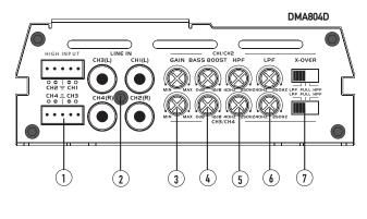
1High-Level Inputs (Speaker Wire)5High-Pass Filter2Line In / Line Out (RCA)6Low-Pass Filter3Gain7Crossover Control4Bass Boost7Crossover Control
