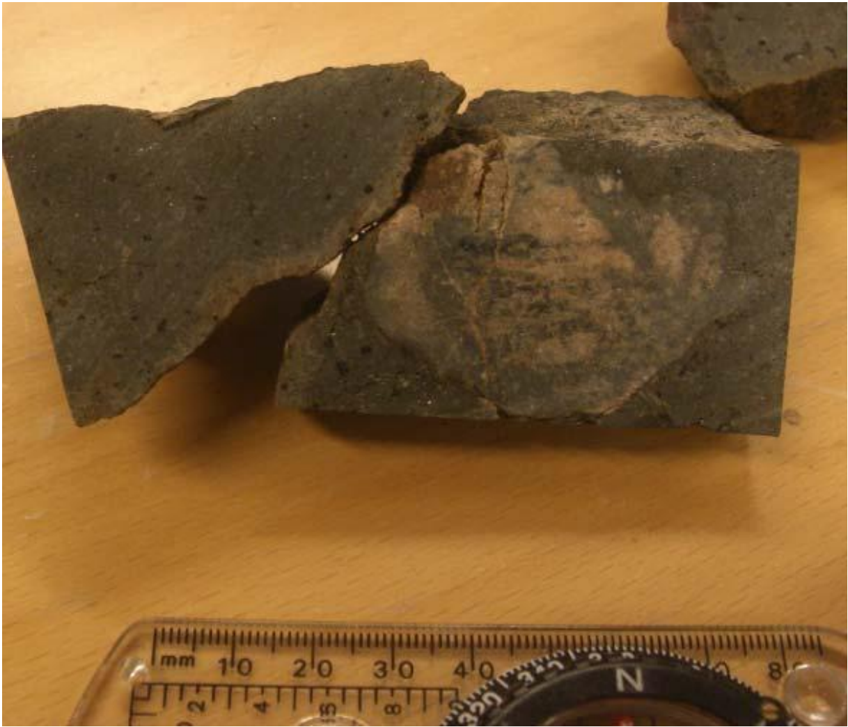
Figure 5-8: Sample from dyke DEF 08-05/DEF 08-06 with a xenolith rich in feldspar. A cm scale can be seen at the bottom.
