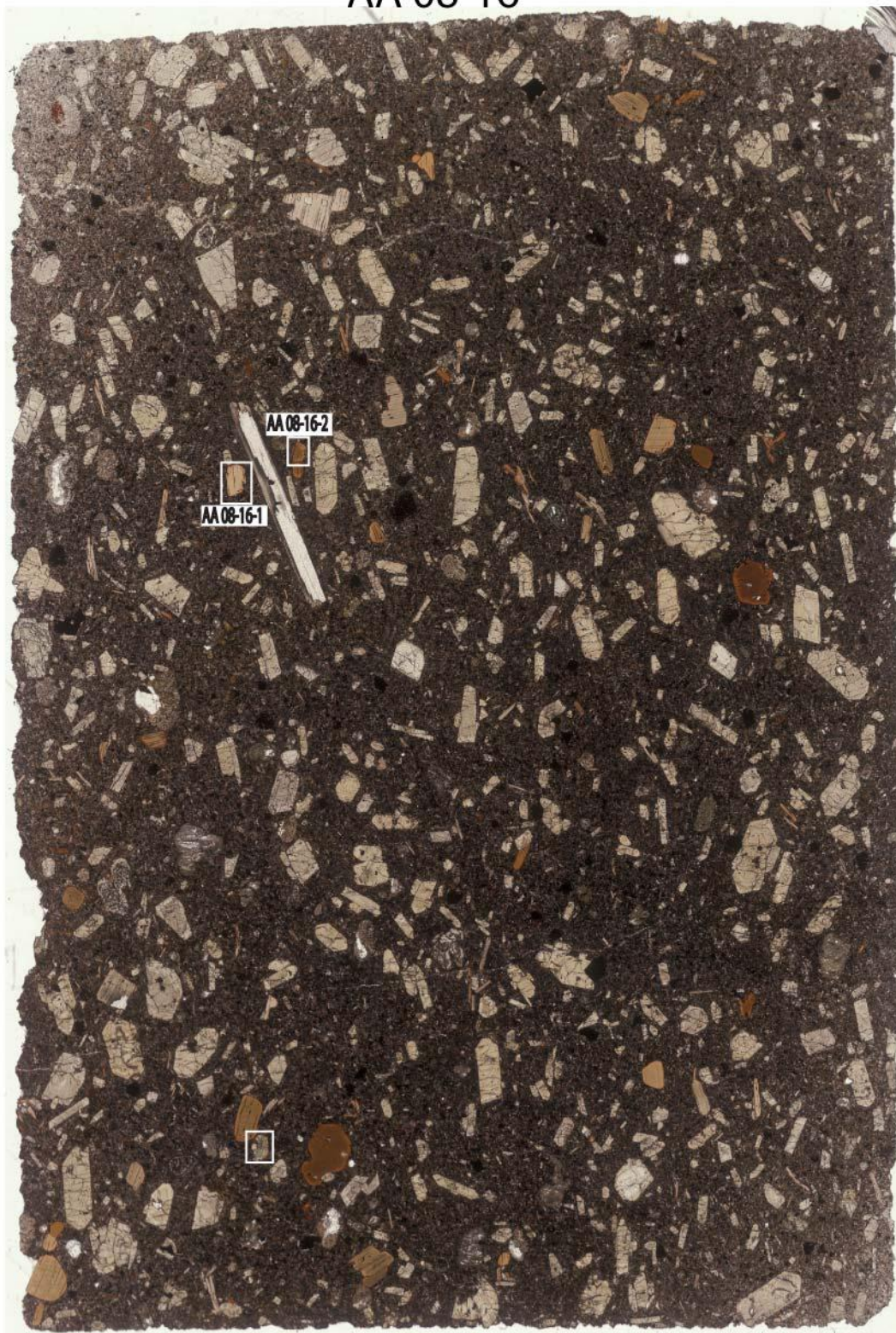
Figure 6-5: Thin-section scan of sample AA 08-16 which is classified as a sannaitite. Phenocrysts of CPX, biotite, spinel, and calcite in a fine grained matrix of CPX, biotite, spinel, K-feldspar, analcite, and carbonate. Biotite phenocryst profiles AA 08-16-1 and AA 08-16-2 can be seen in Figure 8-21, Figure 8-22, Figure 8-25 and Figure 8-26.
