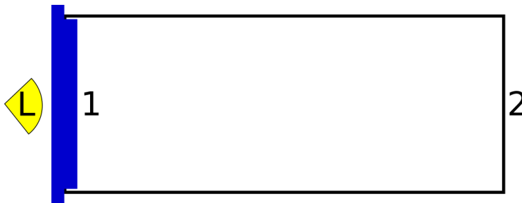
Figura 4: Experimental tank. Blue depicts the lid that close the tank. L is the light source. Light was measured at position 1 and 2.
