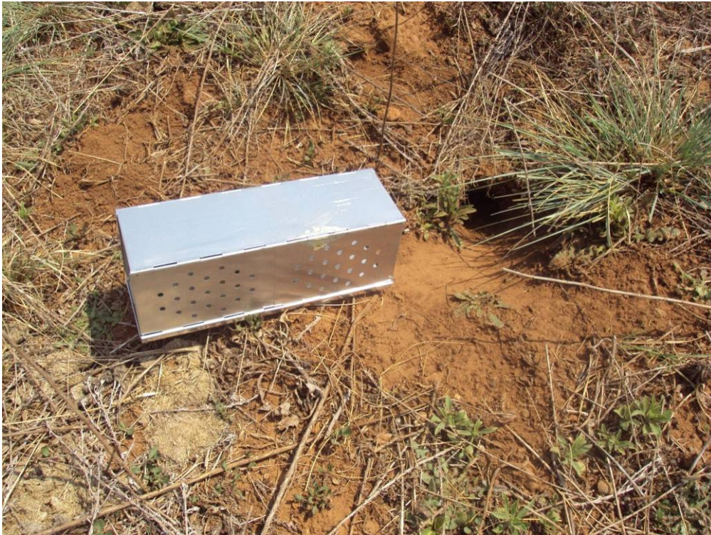
Figure 12. Sherman traps used for small mammals such as rats and mice
