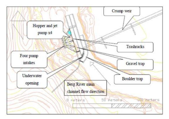
Figure 11: Components of the Proposed Abstraction Works (DWA, 2012)
