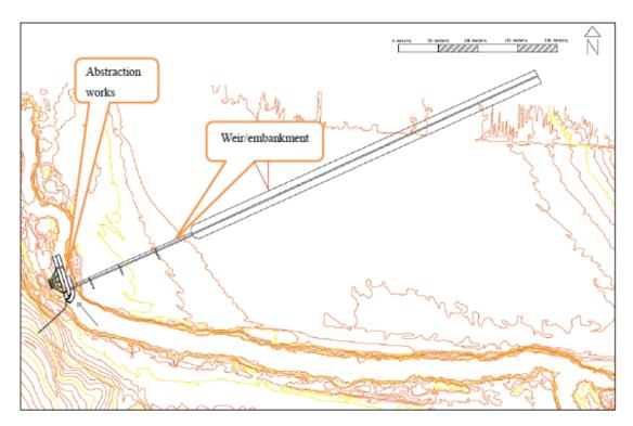
Figure 10: Layout of Abstraction Works, Weir and Embankment (DWA, 2012)
