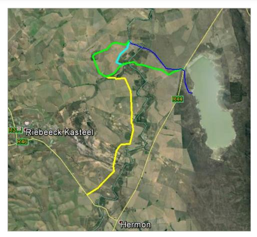
Figure 16: Access road highlighted in yellow to be used during flooding.
