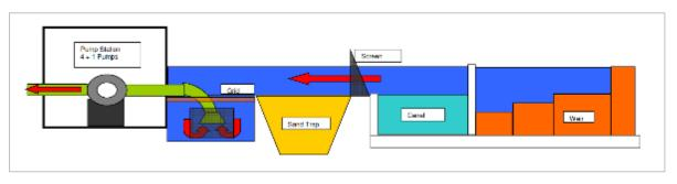
Figure 13: Abstraction point at the proposed pump station
