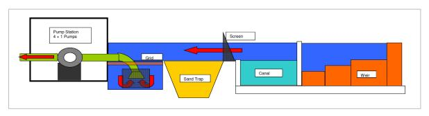
Figure 16: Abstraction point at the proposed pump station
