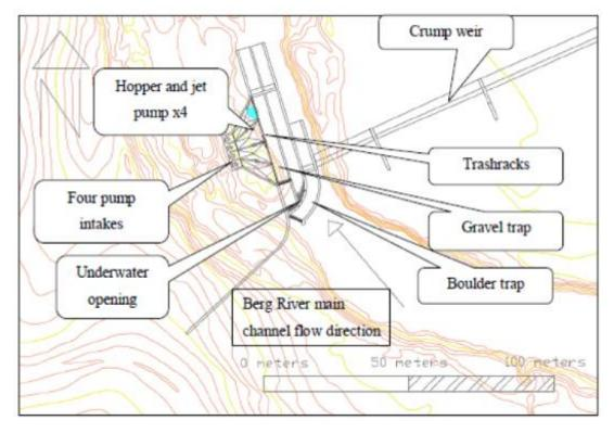
Figure 14: Components of the Proposed Abstraction Works (DWA, 2012)
