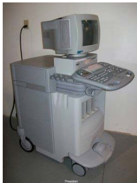
Fig. 14. "Old" ultrasound system. Note the massive size, rendering transport relatively difficult and the "old style" monitor that can be only minimally moved.
