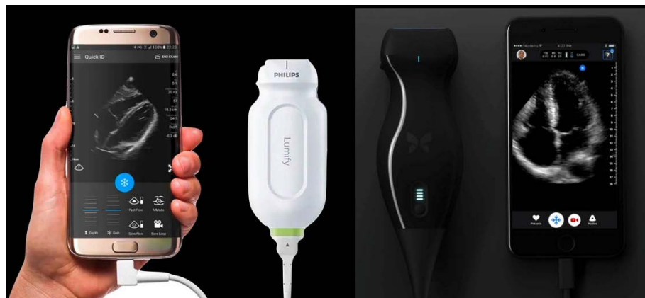
Fig. 18. Two systems using smart phones as monitors. This is a further advancement with the probe attaching directly to a cell phone. One only need to download the application.
