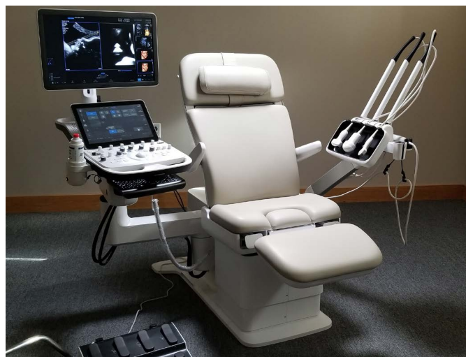
Fig. 8. "Deconstructed" and "reconstructed" ultrasound system. This is an example of a "revolutionary" concept of separating various elements of the ultrasound system. The probes are on one side (right) of the examination chair with a probe holder with recoiling cables while the monitor and keyboard are on the other side (left) of the chair and the actual CPU under the chair.
