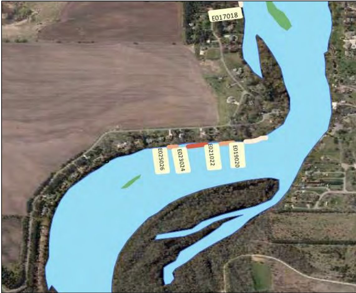
Figure 21: Mississippi River – Sartell Pool sites with defined erosion rates. Note: site E023024 has the third highest erosion rate (Table 4)
