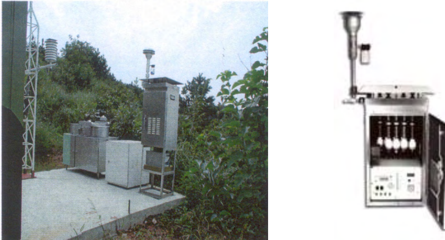
URG (3 stage PM 2.5 Sequential Sampler, USA) Figure 9.14 Instruments used for Dry deposition monitoring
