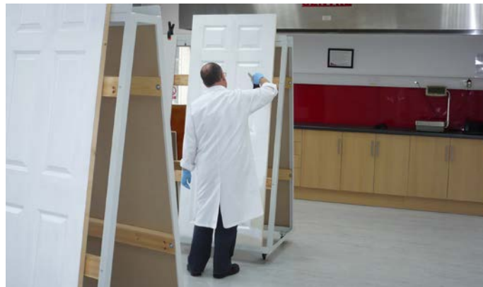
Panel doors are coated with Optifilm OT1200 in preparation for testing.
