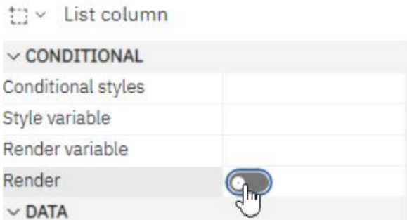
Figure 398 - Hide column in reports -List column properties - Conditional - Set Render to No
