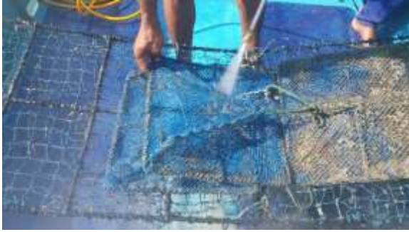
Figure 5-10 Cleaning triangle nets using high pressure cleaner
