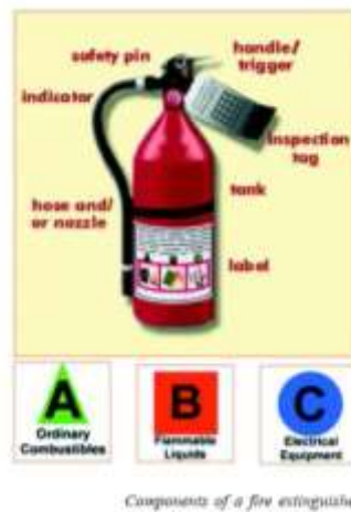
Figure 8-4 Components of a Fire Extinguisher
