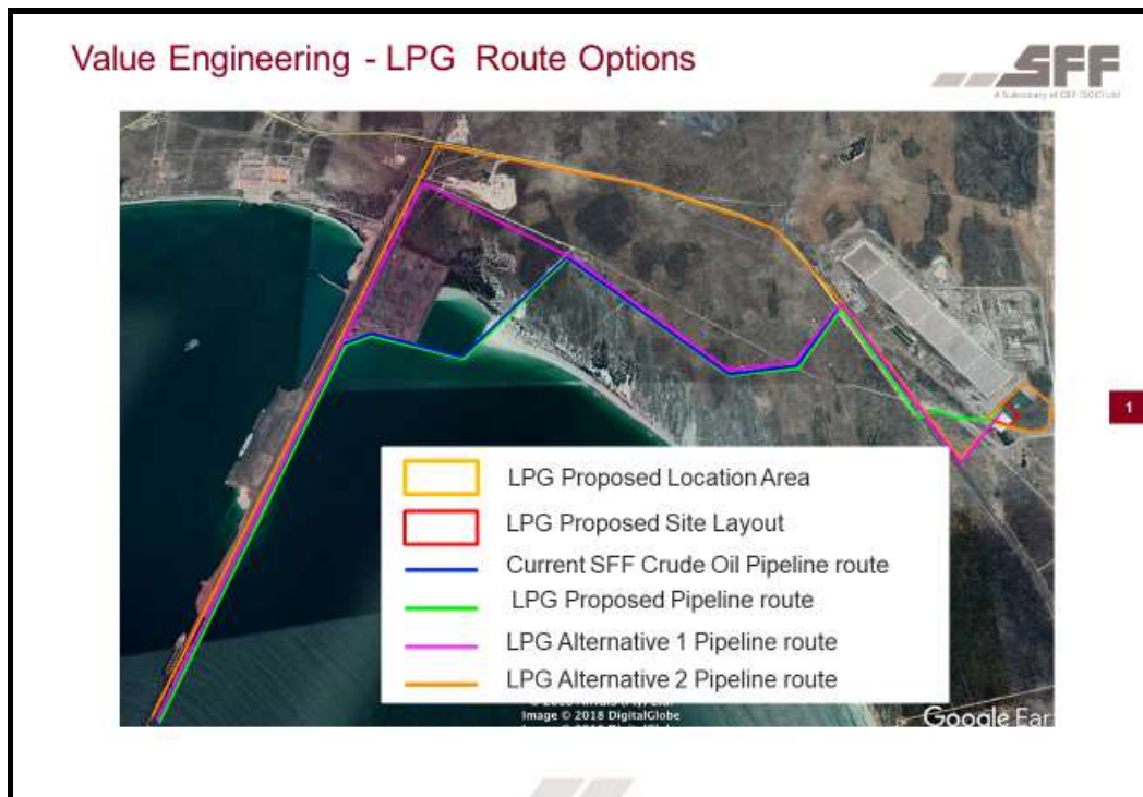
Figure 1: Map showing the three alternative pipeline routes assessed, plus the facility location (see Figure 1b for both facility site alternatives).
