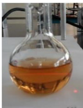
Figure 2 Dissolution of silver nanoparticles prepared with Dandelion extract at pH = 8
