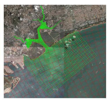
Figure 8.7 Marina Bay 3D model (green grid) and the SIM (red),on the south-central side of Singapore Island
