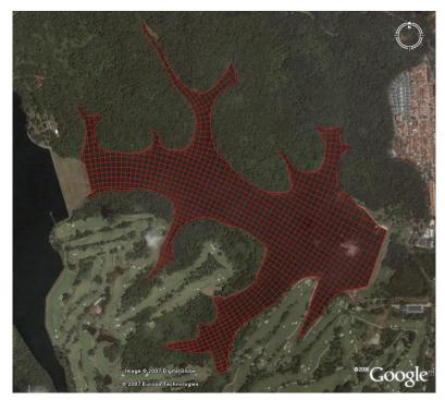
Figure 8.9 Lower Peirce Reservoir model grid
