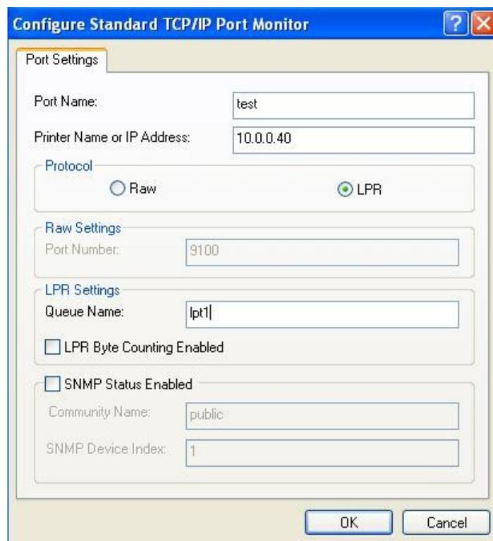
7. This is the setting window when you click on setting on the previous device type settings. The port name and the IP address would be pre-entered for you from the previous settings. At the protocol line, choose LPR and then you will be able to type in LPR settings. Type lpt1 on the queue name and press OK.
