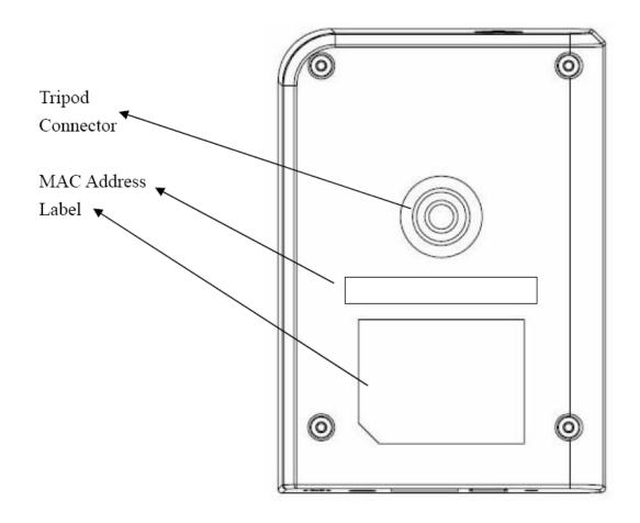
Tripod Connector: Connects to any standard tripod / camera wall holder. MAC Address Label: Shows the MAC address of this Network Camera. Useful when you can't locate the camera on the network.
