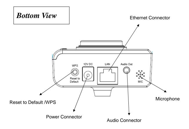
WPS: click the button on IP Cam and click it on the AP you want to connect wireless connection.(works on wired model with USB wifi dongle plugged or wireless model)
