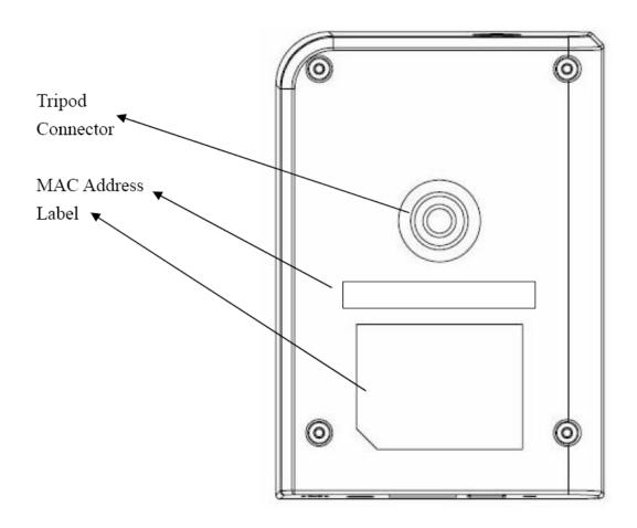
Tripod Connector: Connects to any standard tripod / camera wall holder.
