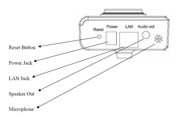
Reset Button: Press and hold for 5 seconds to reset the camera settings to factory default value.
