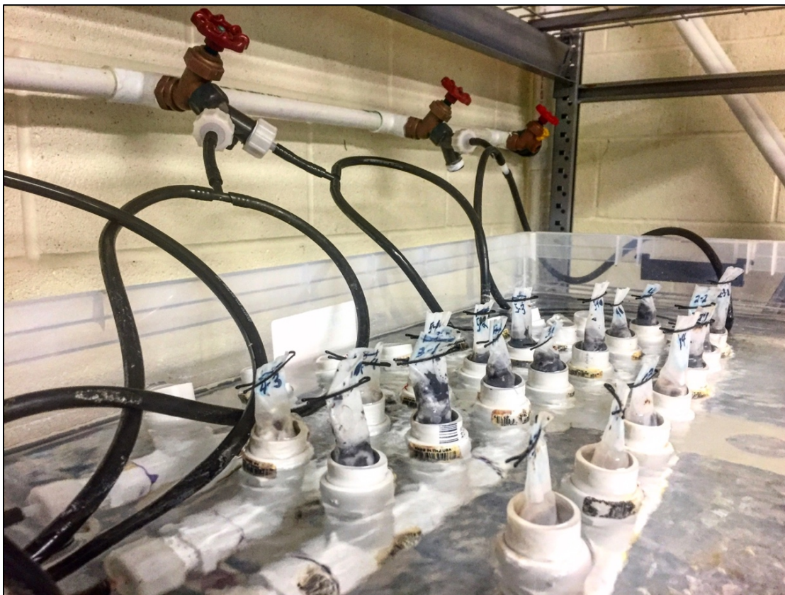
Figure 4. Flow-through upwelling system in use with mesh inserts.
