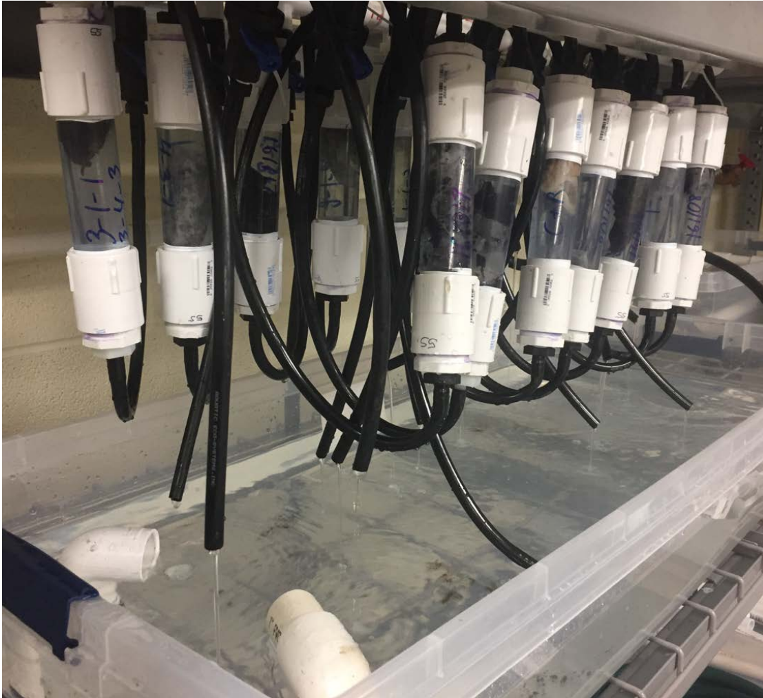
Figure 17. Flow through tubes with flow direction going upward from the bottom and out the top, then captured in the basin below. This system was designed to house cylindrical arrays of substrate intended to mimic in situ conditions likely to promote pupation.
