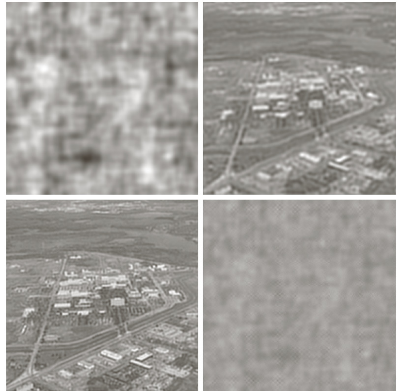
FIGURE 5.27 Restoring Fig. 5.25(b) with Eq. (5.7-1). (a) Result of using the full filter. (b) Result with H cut off outside a radius of 40; (c) outside a radius of 70; and (d) outside a radius of 85.
