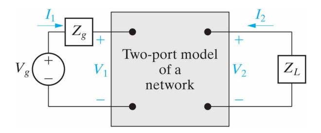
The goal is to solve  $\{V_1, I_1, V_2, I_2\}$  as functions of given parameters  $V_g, Z_g, Z_L$ , and matrix elements of the two-port circuit.
