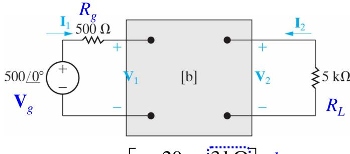
$$[B] = \begin{bmatrix} -20 & 3 k\Omega & -b_{12} \\ -2 \text{ mS} & 0.2 & -b_{22} \end{bmatrix}$$
