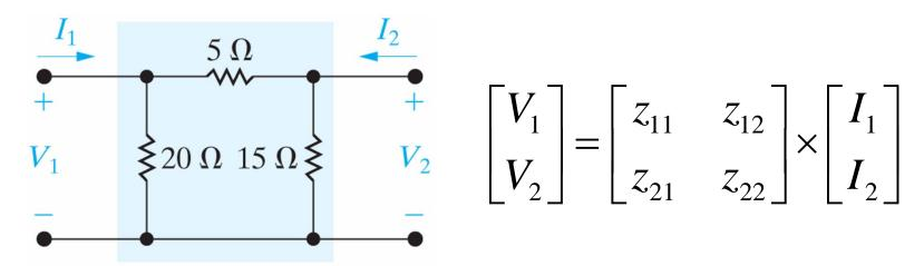
■ By definition,  $z_{11} = (V_1/I_1)$  when  $I_2 = 0$ , i.e. the input impedance when port 2 is open.  $\Rightarrow z_{11} = (20 \ \Omega)//(20 \ \Omega) = 10 \ \Omega$ .
