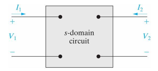
■ Any 2 out of the 4 variables  $\{V_1, I_1, V_2, I_2\}$  can be determined by the other 2 variables and 2 simultaneous equations.
