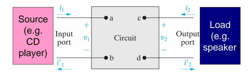
We will see that a two-port circuit can be modeled by a 2×2 matrix to relate the v/i variables, where the four matrix elements can be obtained by performing 2 experiments.
