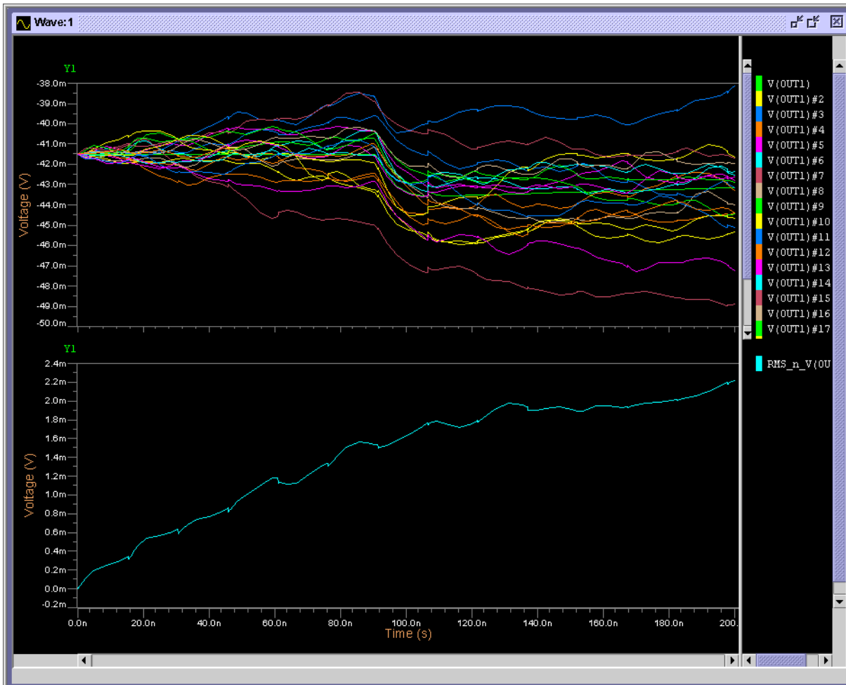
Figure 12-4. Noise at Amplifier O/P
