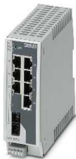
7 RJ45-Ports und 1 LWL-Port (Singlemode)
