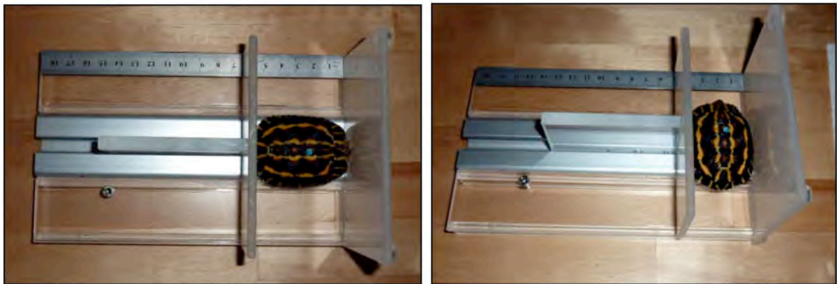
Fig. 32 Calipers used within the EHAP project to measure Pyxis planicauda .
