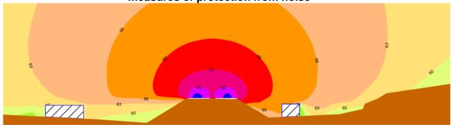
Illustration 6.3.11.4. Cross section of the embankment with noise contours and panel for protection from noise
