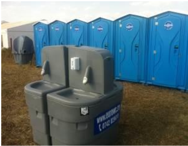
Figure 9.7: Portable chemical toilets and wash basins with sealed water collection tanks
