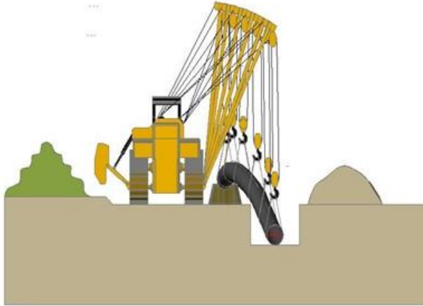
Figure 4.4 Schematic view of gas transmission pipeline laying
