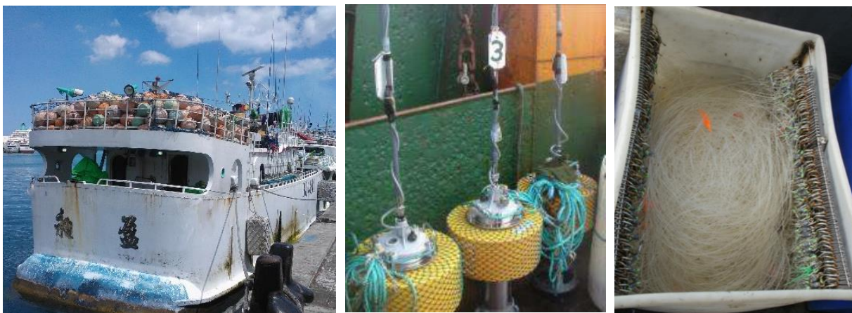
Figure 117: Photographs showing marker buoys (left), radio buoys (centre) and monofilament branch lines (right) (Source: CapMarine, 2015).
