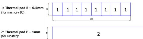
4. PLACING THERMAL PADS ON PCB. Place thermal pads on the circuit board as shown on the picture below. Refer to numbering in previous picture when applying thermal pads of different sizes or thicknesses. EK made sure to provide customers with more than adequate quantity of thermal pads to complete this step.
