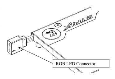
Plug the 4-pin connector from Water block's RGB LED light to the RGB\_HEADER on the motherboard. The LED will work if the pin layout on the header is as follows: <u>+12V G R B</u>.
