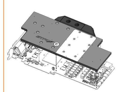
2. ATTACHING THE BLOCK TO THE GRAPHIC CARD. Use a Philips screwdriver screw with the enclosed M2,5x4 AX1 screws. EKWB recommends users to start tightening the screws around the GPU core and continue outwards. <u>Always use</u> a plastic washer under each and every screw! If the washer is already present on the circuit board (usually around the four GPU core screw holes) there is no need for additional washer.
