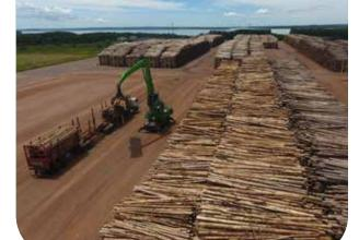
The supplied wood is segregated into piles in the **stockyard**, taking into account factors such as:
