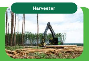
Tree felling, branch and twig removal, bark stripping, and cutting into specified lengths are carried out by harvesters. Log bundles are stored for subsequent transshipment, which usually takes place around 10 days after felling.
