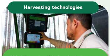
Digital harvesting: Digital technologies are used to monitor harvesting operations, including automatic production cycles, production status, telemetry, and remote sensing of harvesters and forwarders.
